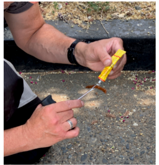
Apply cement to plug
